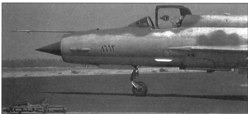
This MiG-21MF, flown by the Soviet 135th Air Regiment in Egypt in 1970-71, displays the camouflage scheme applied at the Gorky factory in Russia. These aircraft received Egyptian national markings and serial numbers, 8692 in this case (Russian military Archives)
